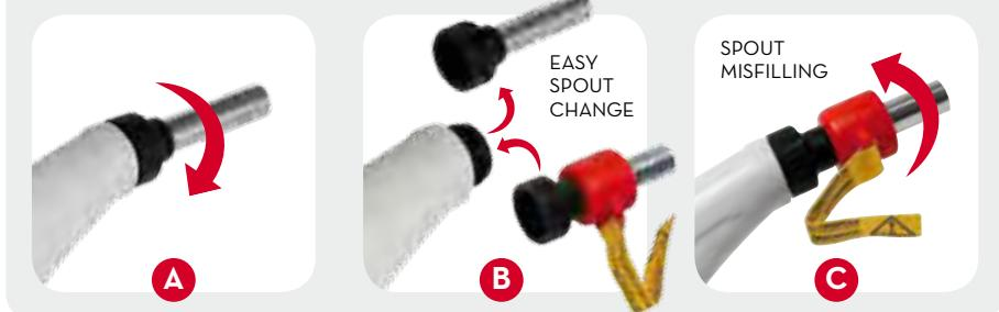
**EN.** Safety is guaranteed by the break-away system. In the event that a vehicle accidentally drives away with the nozzle still in the tank, the spout is designed to detach from the nozzle. This system also allows for a quick repair by merely fitting a new spout onto the nozzle.
