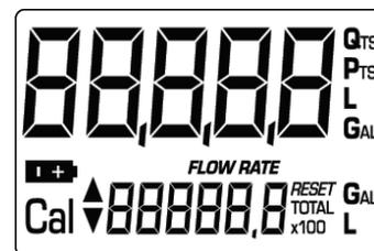
and after a few moments, the Reset Total is replaced by the NON-resettable "Total".
