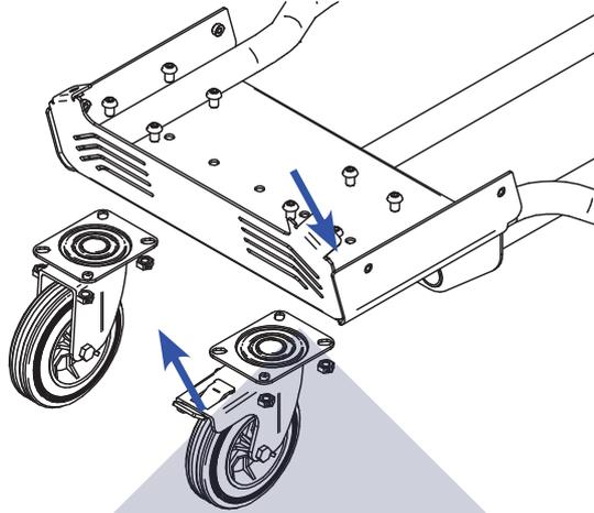
**2 Fitting fixed wheels on drum trolley**
