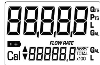
At the end of the process, a screen showing the reset Partial quantity and Reset Total is displayed
