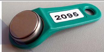
ELECTRONIC KEYS are used by pressing them to the KEY READER located on the MC's front panel.
